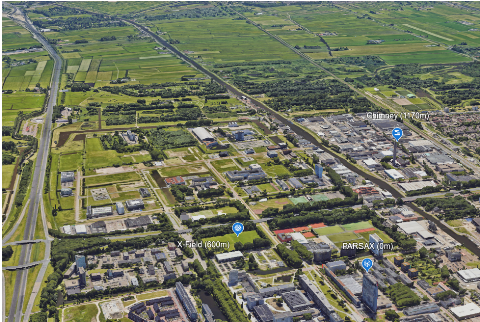
Figure 5.2: Aerial view of the experimental area. PARSAX radar at the origin, chimney target at 1180 m, X-Fields at 600 m.
